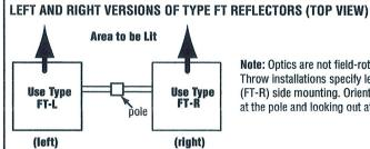
Note: Optics are not field-rotatable. For D180 Forward Throw installations specify left (FT-L) and/or right (FT-R) side mounting. Orientation is based on standing at the pole and looking out at the area to be lit.
